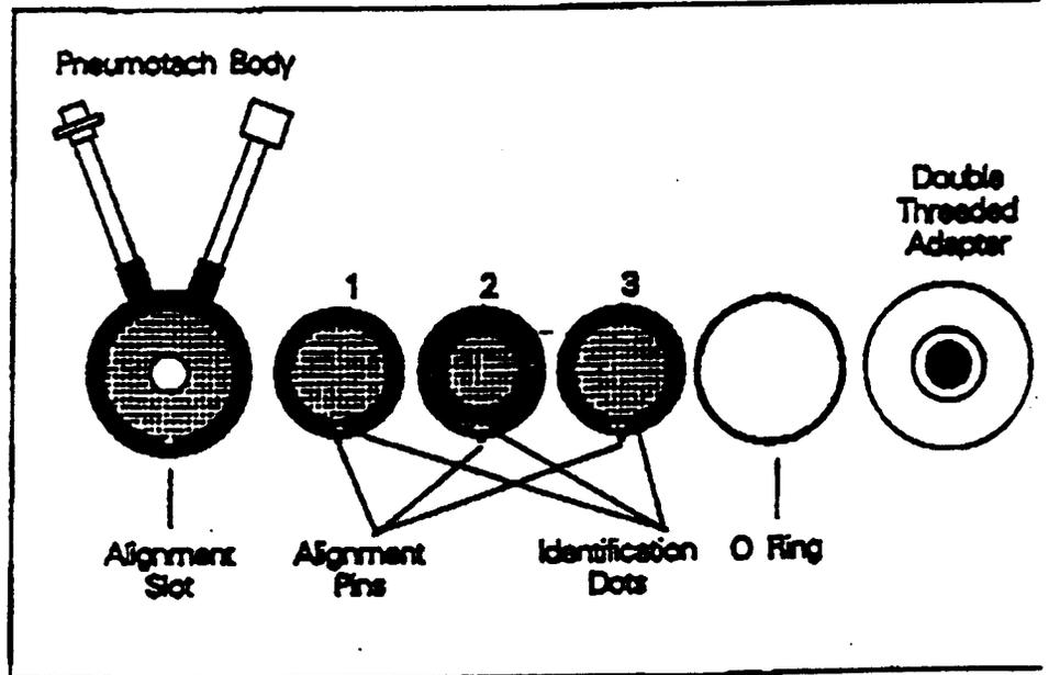
Figure 13.4. Exploded view of 30 LPM Pneumotach.
