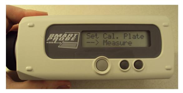
Calibration with the white tile is required each time the device is powered on for use. When the SmartProbe device is turned on and the user is prompted to calibrate the device by the "Set Cal. Plate" screen (above), place the device on the white calibration tile provided and press the primary button (on top side of device) once. A blank calibration measurement screen will appear (below).
