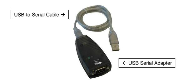
5. Connect the USB serial adapter to the RJ45-to-serial port cable.
