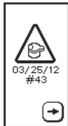
The alert screen will continue to appear until the Sensor has expired. The number of remaining tests on a Sensor will be displayed on the Main screen of the NIOX MINO unit. When this number reaches "0", a new sensor will need to be installed.
