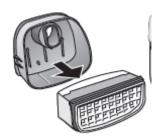
3. Insert the new NO scrubber into the cover. Make sure to use a new NO scrubber with an unbroken hole.
