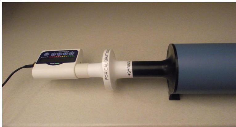
4. Pull the 3-liter piston fully out before beginning the test.
