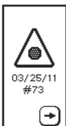
This alert screen is shown when 10% of the measurements are left, or two weeks before the expiration date. The alert screen will continue until the NO scrubber has expired. The number of remaining uses and the date of expiration will be displayed.
