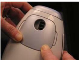
6. Remove black latch from back of power unit and insert correct outlet for plug.
