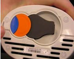
3. Insert the NO scrubber into the back of the instrument. To remove the cover, spread the latches apart, one at a time, and carefully pull out the cover
