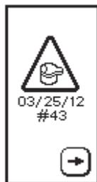
The alert screen will continue to appear until the Sensor has expired. The number of remaining tests on a Sensor will be displayed on the Main screen of the NIOX MINO unit. When this number reaches "0", a new sensor will need to be installed.
