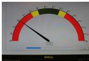
Fig. 2b. Arrow is to the left of green zone. Pressure is too low.
