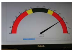
Fig. 2c. Arrow is to the right of the green zone. Pressure is too high.
