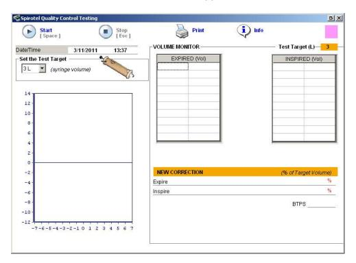
12. Make several complete expirations and inspirations (piston fully out to piston fully in) at different flow rates so that a green indicator bar appears for each expired flow rate and inspired flow rate. When all the flow rates are green, extend the piston fully in and out one more time for the test result to appear.
