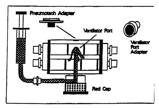
Figure 14.1. Occlusion Valve Cleaning
